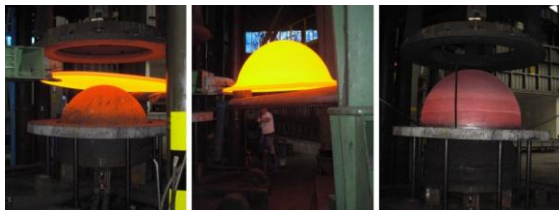
Fig. 4: Deep drawing of one hemispherical dished head of Ictineu 3 pressure hull (courtesy of ATB Riva Calzoni S.p.A.)
