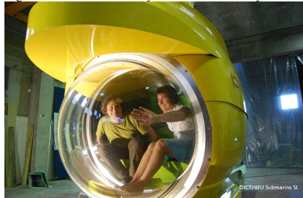
Image of unfinished submersible assembly and detail of visibility in the front acrylic window, in summer 2011.
