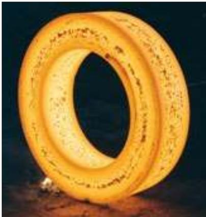
Fig. 4. A forged ring before heat treatment (courtesy of Special Flanges).
