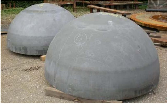
Fig. 3. Hemispherical dished heads of Ictineu 3 pressure hull (courtesy of ATB Riva Calzoni S.p.A.).
