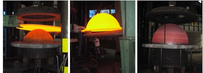
Fig. 2. Deep drawing of one hemispherical dished head of Ictineu 3 pressure hull (courtesy of ATB Riva Calzoni S.p.A.).
