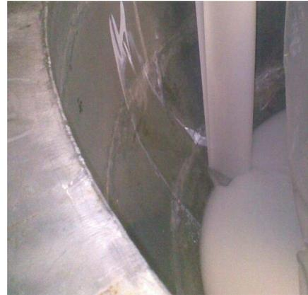
Fig. 6. Acrylic cast of Ictineu 3 window (courtesy of Stanley Plastics).
