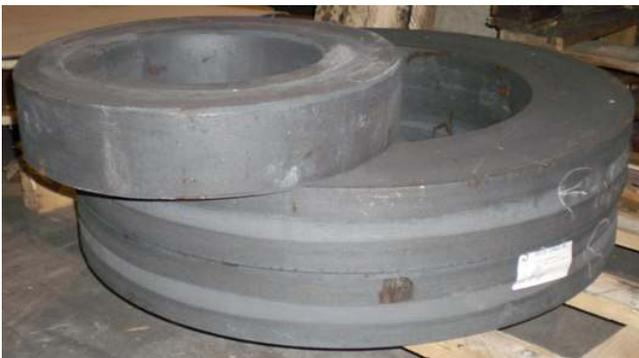
Fig. 5. Forged rings of Ictineu 3 after heat treatment, ready to be machined (courtesy of Special Flanges).
